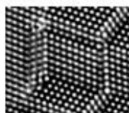
Atoms of silicon spacing ~ tenths of nm
